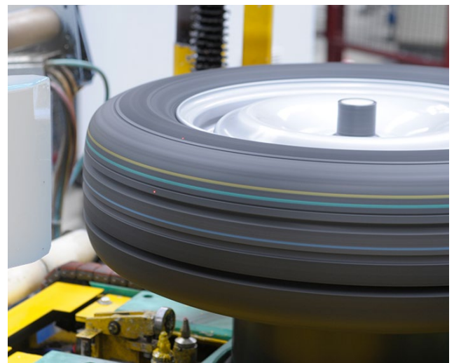
Integration to balancing machine
