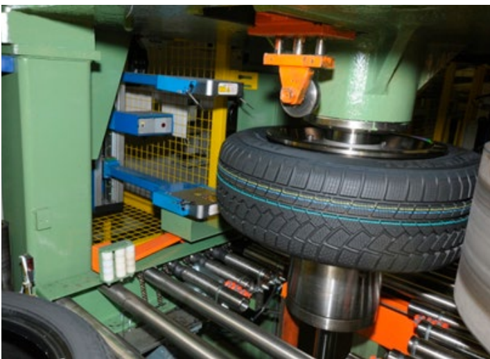
Integration to tire uniformity machine
