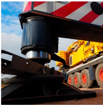
Variable support for mobile cranes
